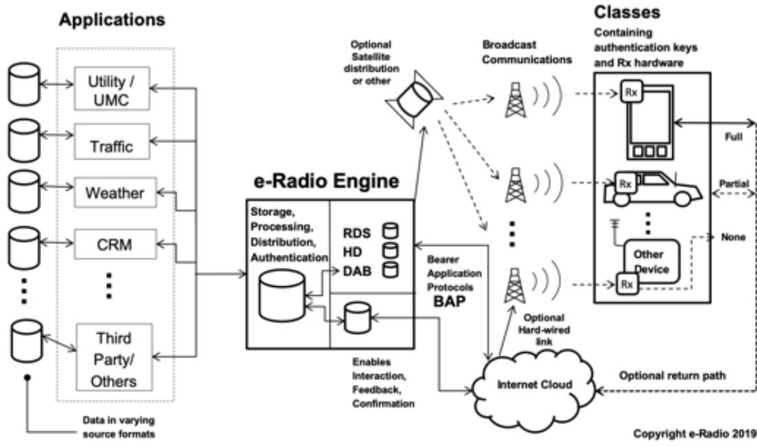
Figure 2. Hybrid IP+FM data architecture
