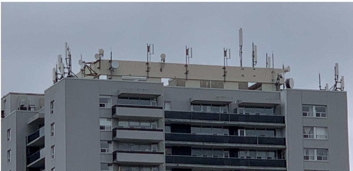
*Fig 11. Sample cellular repeater station atop of a residential building*
