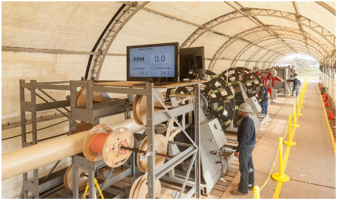
Figure 10. Smart Pipe Company fabricates flexible pipe onsite, in a continuous process, of any length, without joints. Multiple non-ferrous layers may provide adequate H2 permeation barrier without embrittlement; polymer-metal hybrids may be necessary, as in Fig 10. NREL will test H2 permeation and burst; may have time for P cycling.
