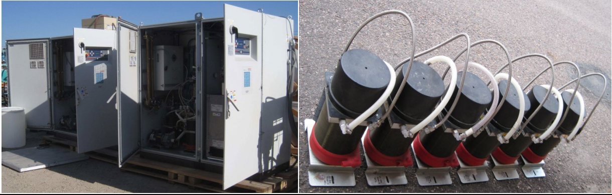
Figure 9. Two used Proton OnSite H6m electrolysis plants; their six electrolysis stacks dedicated to this project. Owned by AASI; in-kind contribution.
