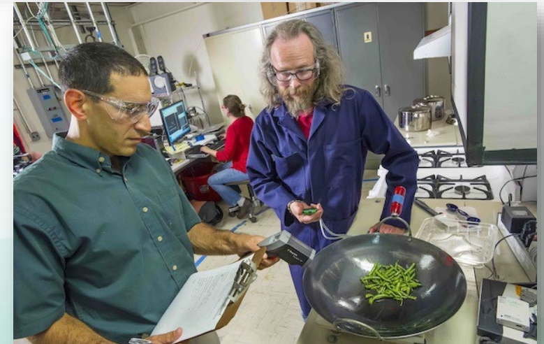
Measuring indoor air quality (source: LBNL)
