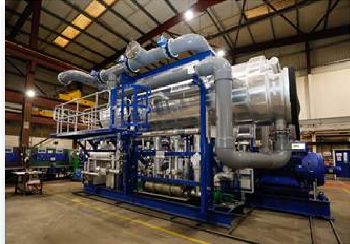
Example of electric heat pump Source: flicker.com
