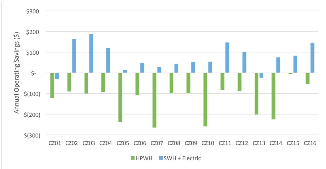
Figure 1. Annual savings realized from operating residential HPWH and SWH + Electric as compared to storage type gas water heaters across California's 16 climate zones<sup>8</sup>
