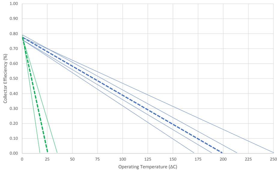
Figure 27. SRCC OG-100 collector efficiency curves for glazed selective surface (blue) & unglazed polymer (green) under full sun ( $1000 \text{ W/m}^2$ ). Individual sample collectors are shown as light solid lines. Average collector performance used in simulations is illustrated by the thick dashed lines.
