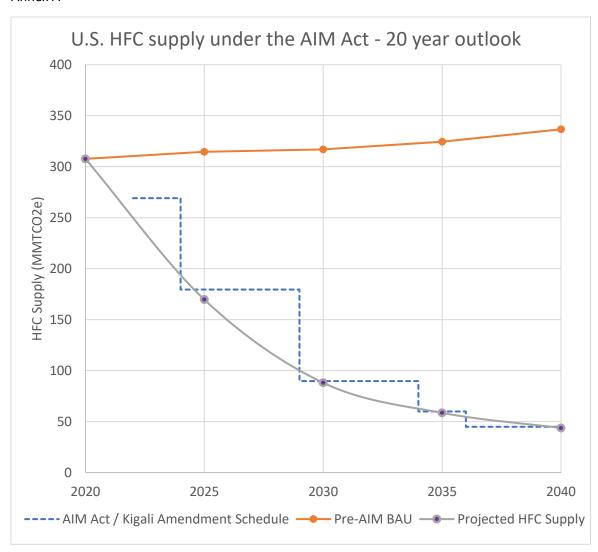
Source: NRDC analysis of EPA data under the AIM Act allocation rulemaking, 2021. Note: the "Projected HFC Supply" curve is required to stay *under* the "AIM Act/Kigali Amendment Schedule." The "Projected HFC Supply" data points are connected by a curved line for visual effect only; data for intervening years has not been estimated.
