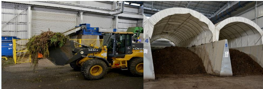
Example of green waste feedstock (left) and digestate (right). (Credit: HZIU Kompogas)
