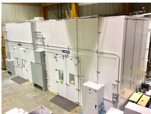
LBNL Psychrometric Test Chamber
