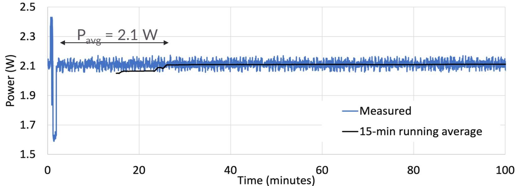
*Example of test period for a connected smart home product that powers down to a pinging mode. Preliminary data for illustration purposes only. Source: CA IOU Team.*
