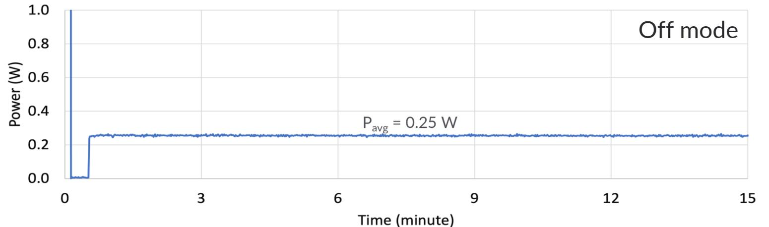
Example of additional tests for a game console: manual power down (top) and off mode (bottom). Preliminary data for illustration purposes only. Source: CA IOU Team.
