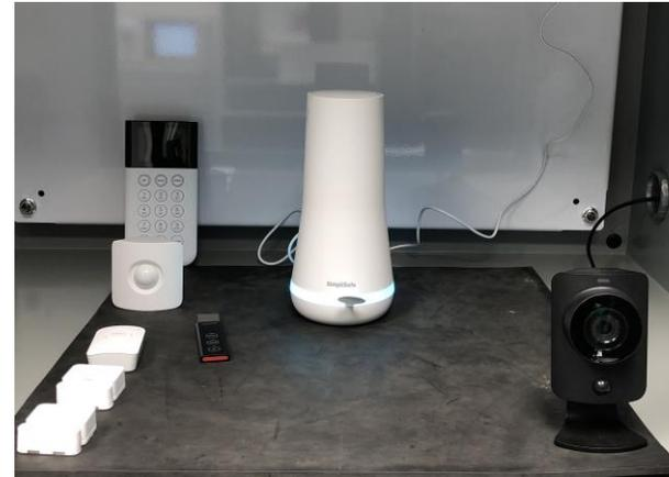
Connect base station and camera to 120Vac power
