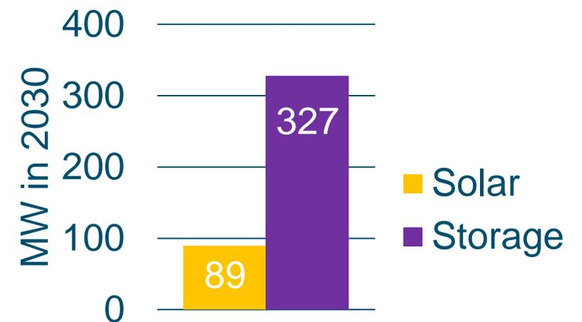
Additional solar and storage required in 2030 for unmanaged EV charging shape
