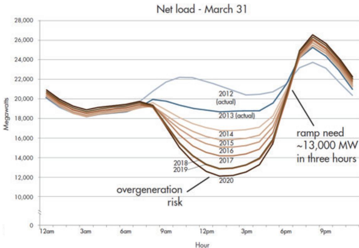
**FIGURE 7.5** Projected daily electricity demand, minus wind and solar generation, on a typical spring day in California. There is a risk of overgeneration in the middle of the day and early afternoon, followed by a steep ramp where an additional 13 GWe is needed. Credit: California Energy Commission (2017), Figure ES-4.
