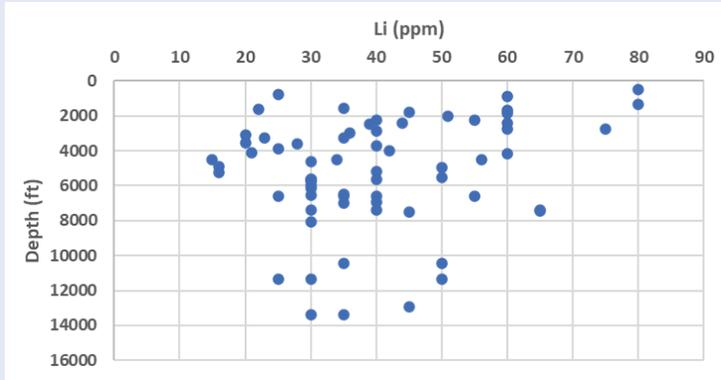
**FIGURE 7.3** Variation of lithium (Li) metal content in parts per million (ppm) versus depth for cuttings and core from several drill holes in the Salton Sea Geothermal Field. Credit: Mike McKibben. Source: Unpublished spectrographic data provided to S. D. McDowell, collected in 1971 by D. E. White, L. J. P. Muffler and H. Bastron, USGS.
