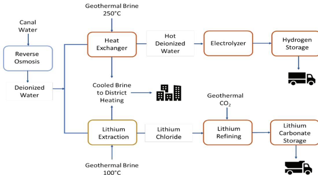
**FIGURE 7.6** Conceptual design of lithium and hydrogen extraction from Salton Sea geothermal brines at temperatures of  $250^{\circ}\text{C}$  and  $100^{\circ}\text{C}$ . Direct conversion of lithium chloride to a lithium hydroxide product would be more advantageous for battery manufacture. Credit: Elders et al. (2019).
