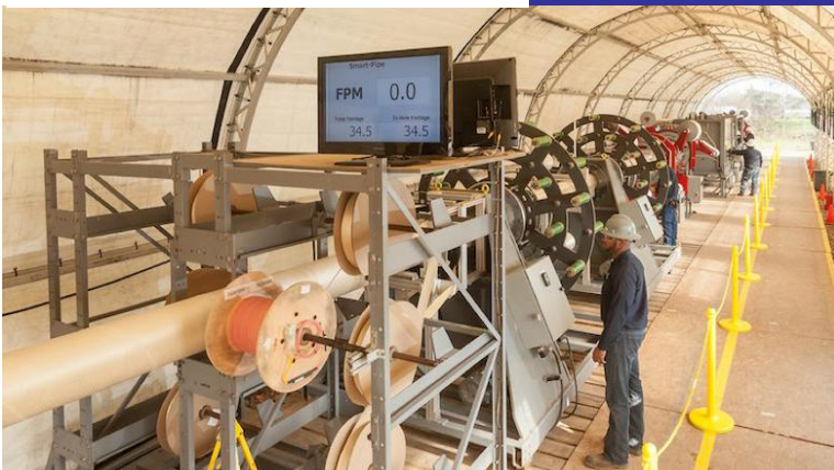
Smart Pipe Company, Houston On-site pipeline factory Continuous process, unlimited length Hydrogen-compatible: polymer-metal hybrid resists HE, HCC
