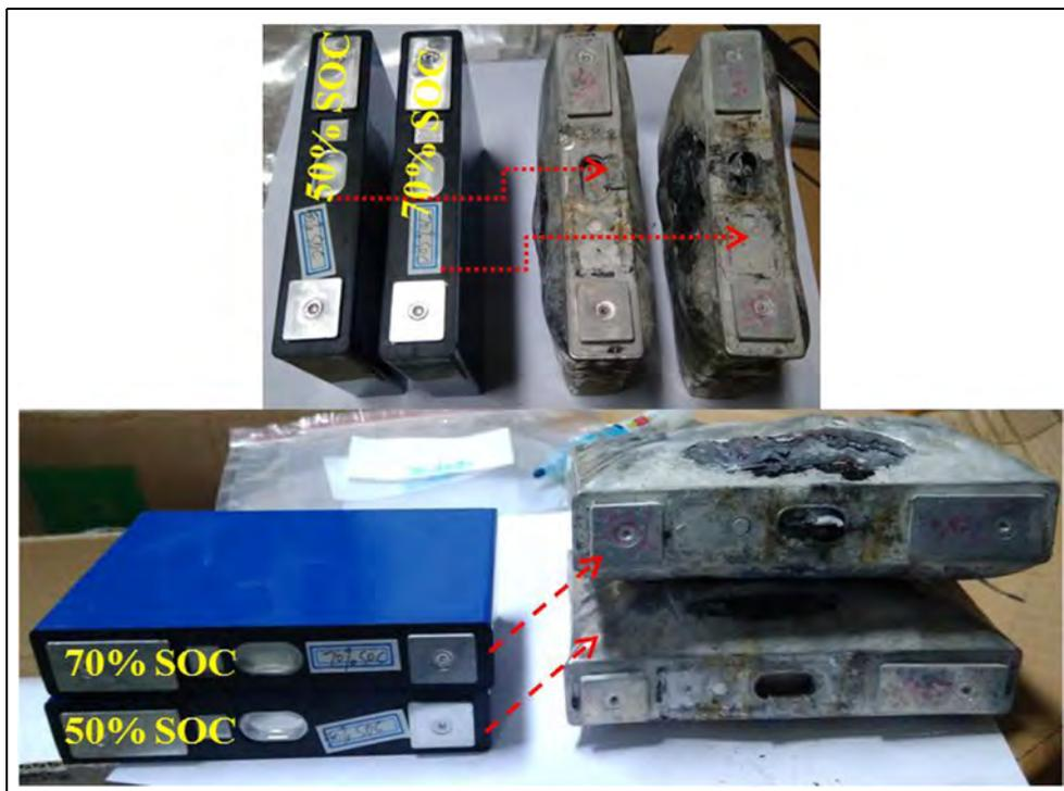
**Figure 11.** The images of LIBs before and after thermal failure.
