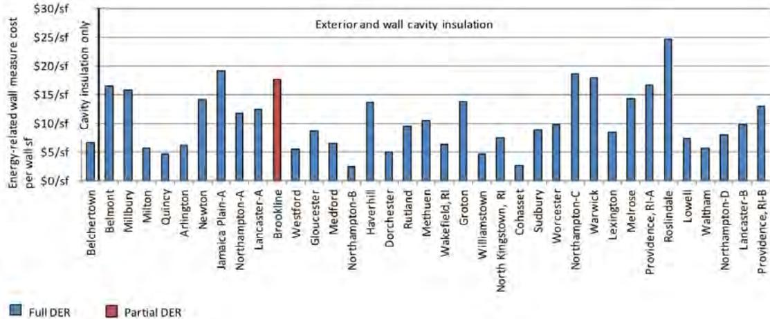
Figure 15 Total energy related exterior wall costa per wall ft<sup>2</sup> (Gates and Neuhauser, 2014)
