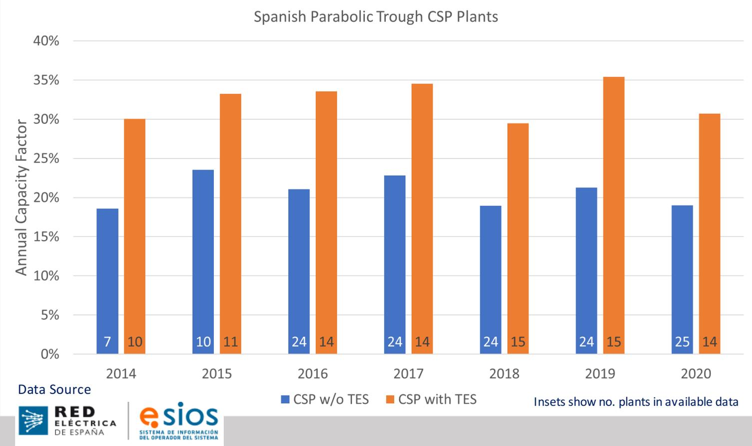
In the Spanish market and climate, trough plants with no TES are typically designed for about 20% annual capacity factor, while 30% to 35% is the corresponding target capacity factor for plants with 7 to 9 hours of TES.
