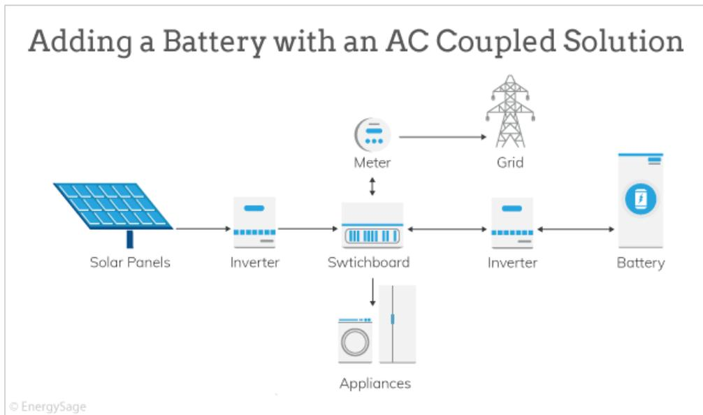
**Figure 2: Battery storage system paired with solar PV.**
