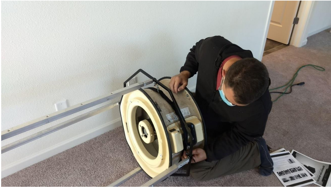
Figure 5: The PFH uses a standard fan flowmeter to measure airflow.
