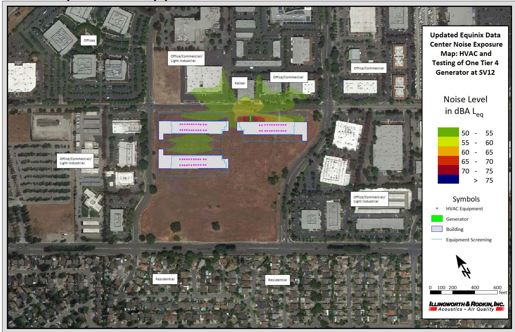
FIGURE 1 Noise Exposure Resulting from Testing of One Generator at Building SV12 at 100% Load Concurrent with Operation of HVAC Equipment
