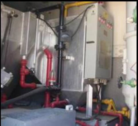
Electrolysis to Precipitate Solids
