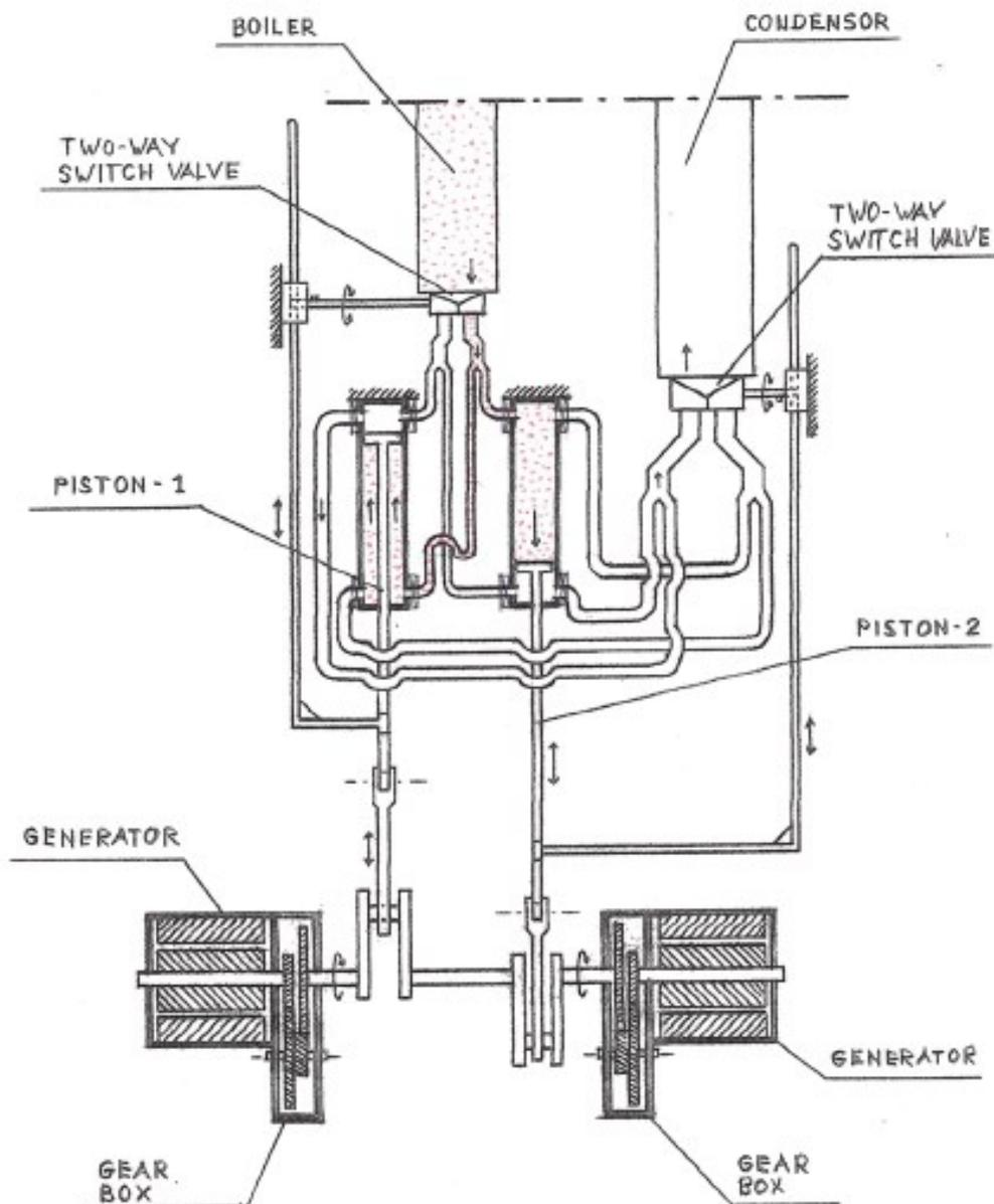
**FIG. 9** – Schematic Diagram of a Piston Power Unit –
