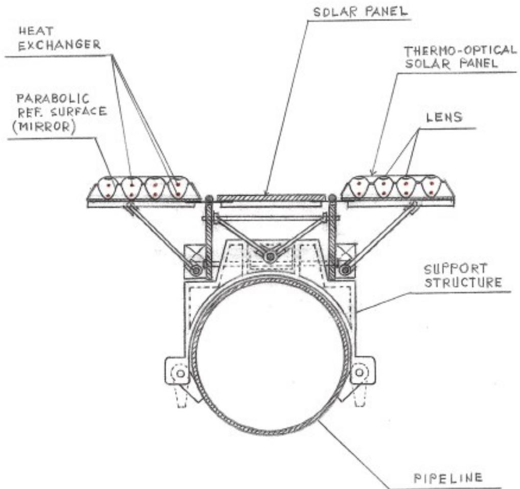
**FIG. 2** – Cross-sectional View of a Solar Panel Assembly
