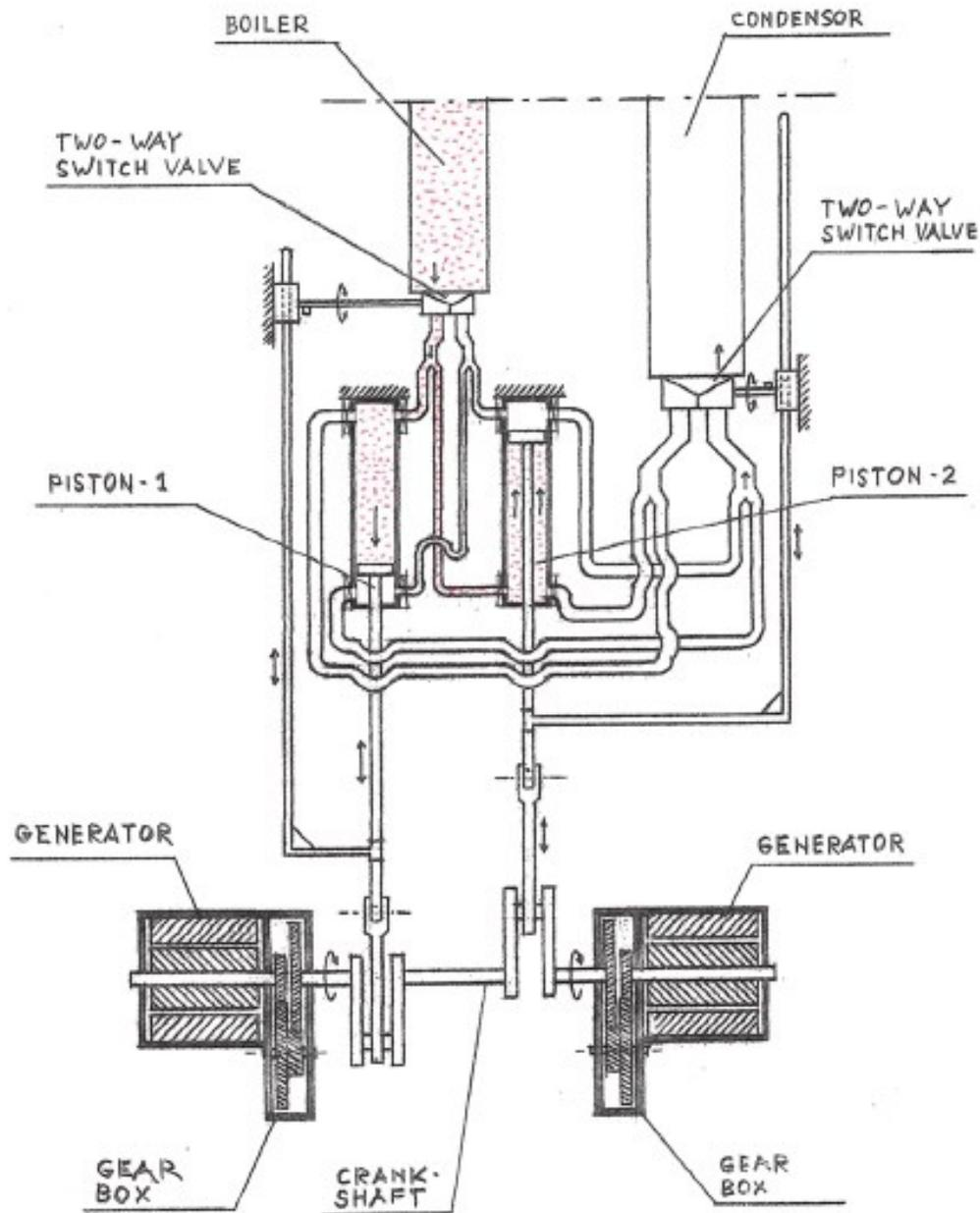
**FIG. 8** – Schematic Diagram of a Piston Power Unit
