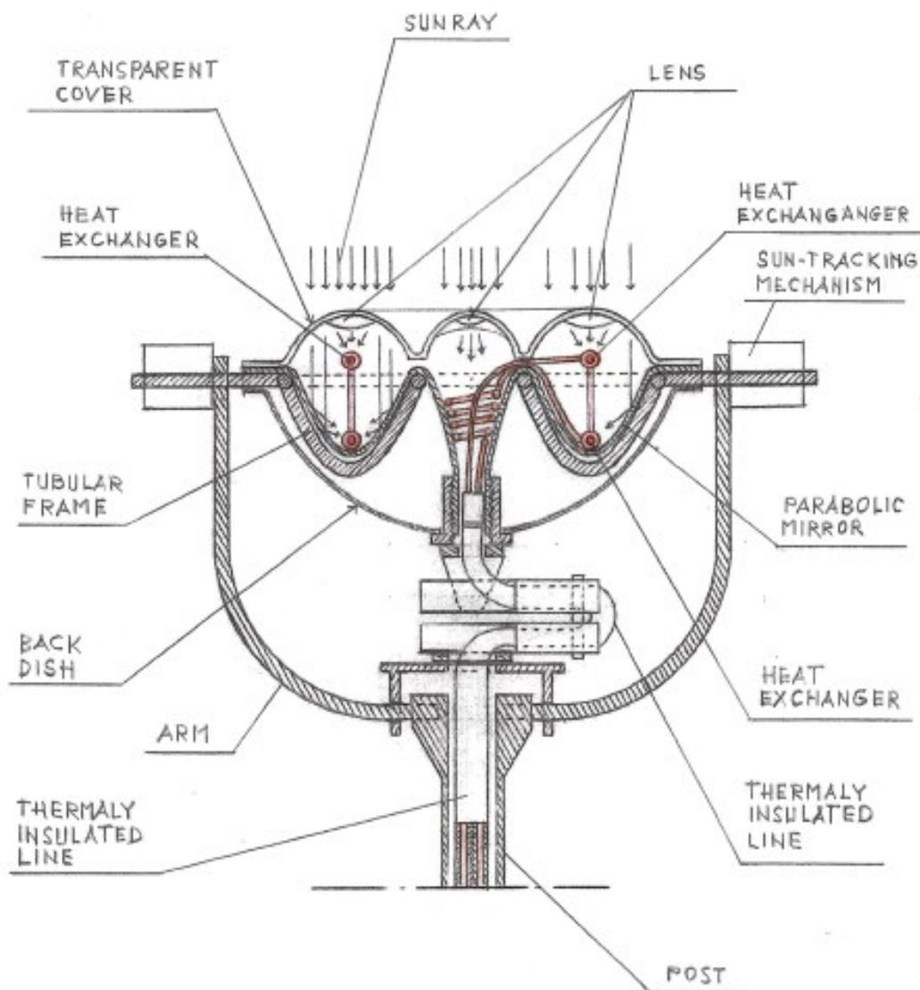
**FIG. 3** – Cross-sectional View of the "Thermo-Optical Solar Dish"
