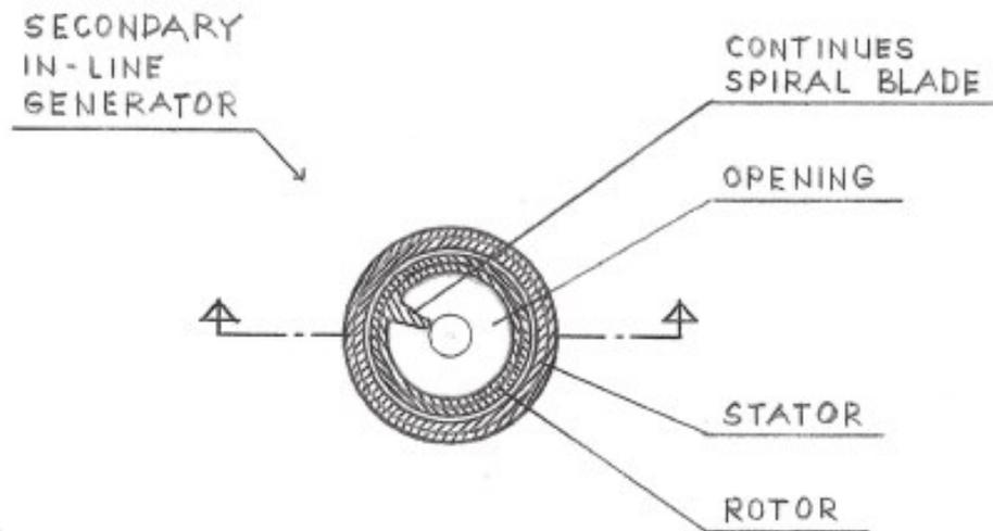
**FIG. 8** – Cross-sectional Frontal View of the Primary and Secondary In-Line-Pump / Generator
