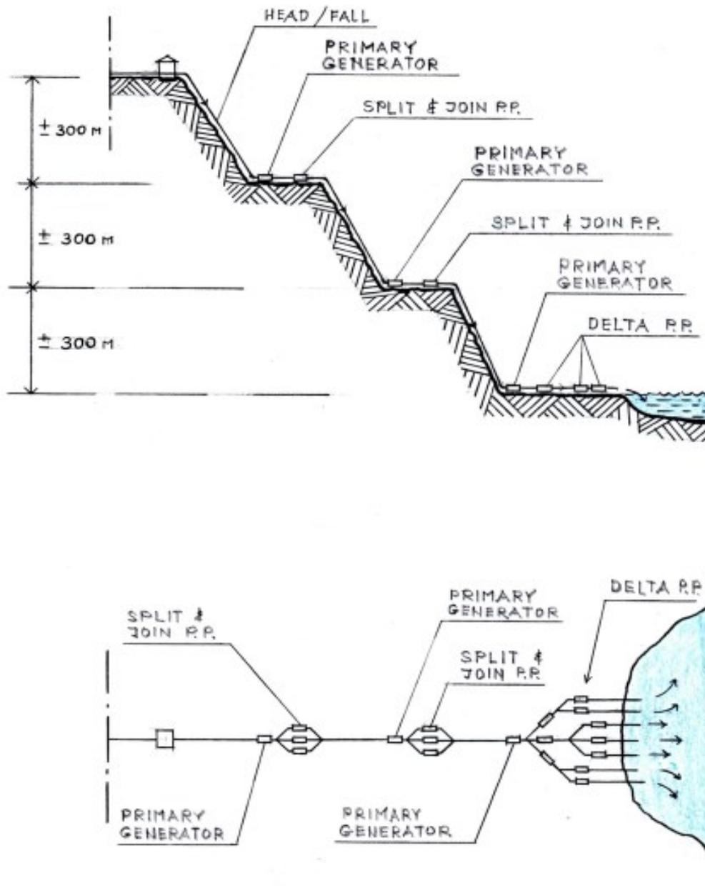
**FIG. 5** – Plain and Cross-sectional View of the final downhill route
