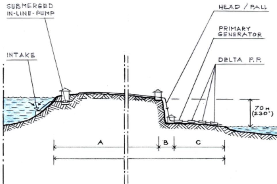
**FIG. 2** – Cross-sectional View of the Route #1
