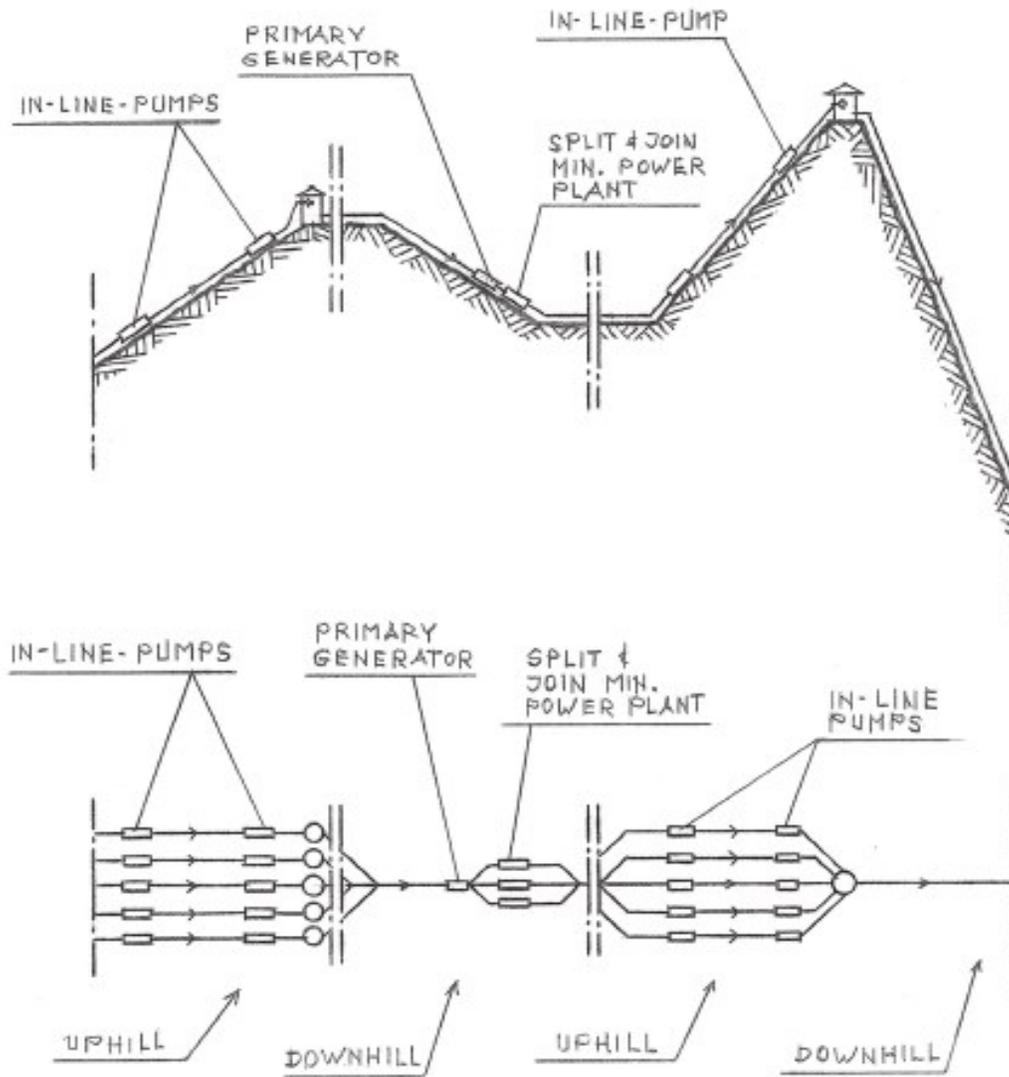
**FIG. 4** – Plain and Cross-sectional View of the Mid-section of the Pipeline
