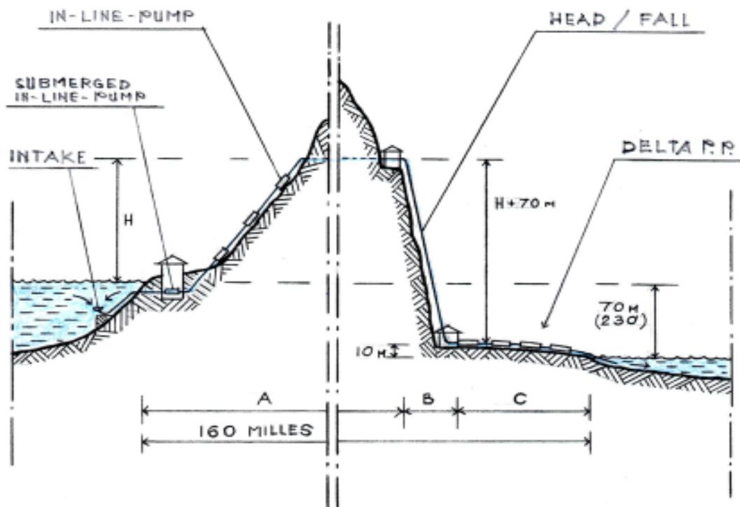
**FIG. 3** – Cross-sectional View of Elevations of the Ocean and Salton Sea
