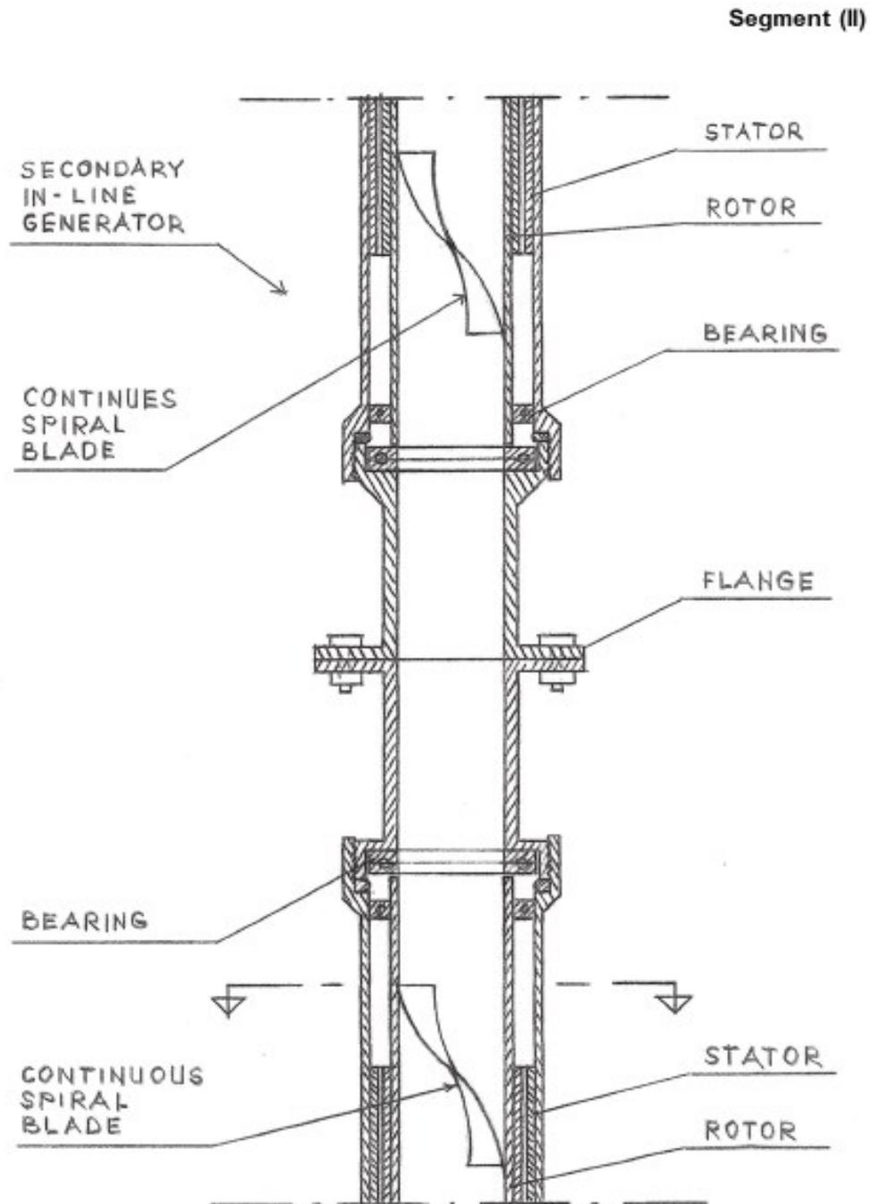
**FIG. 7 – Cross-sectional longitudinal View of the Secondary In-Line-Pump/ Generator**
