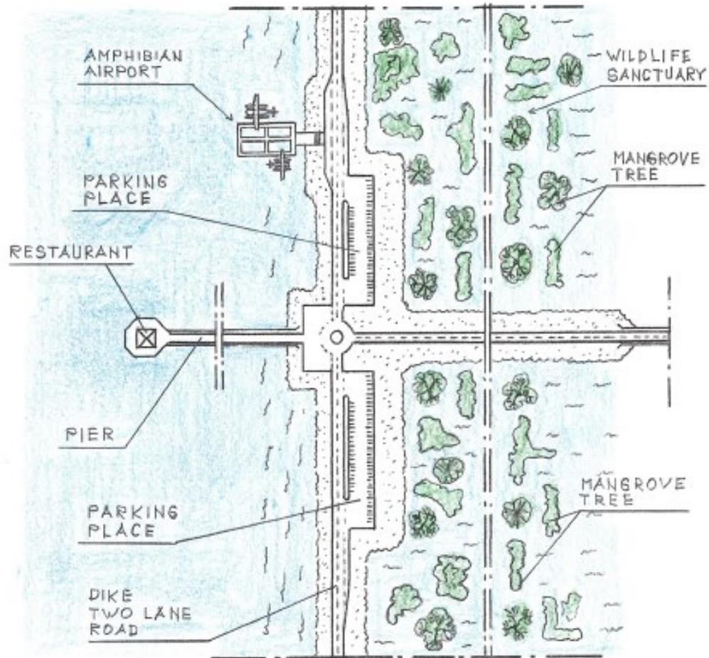
**FIG. 7** – Plain view of a typical dike-pier intersection
