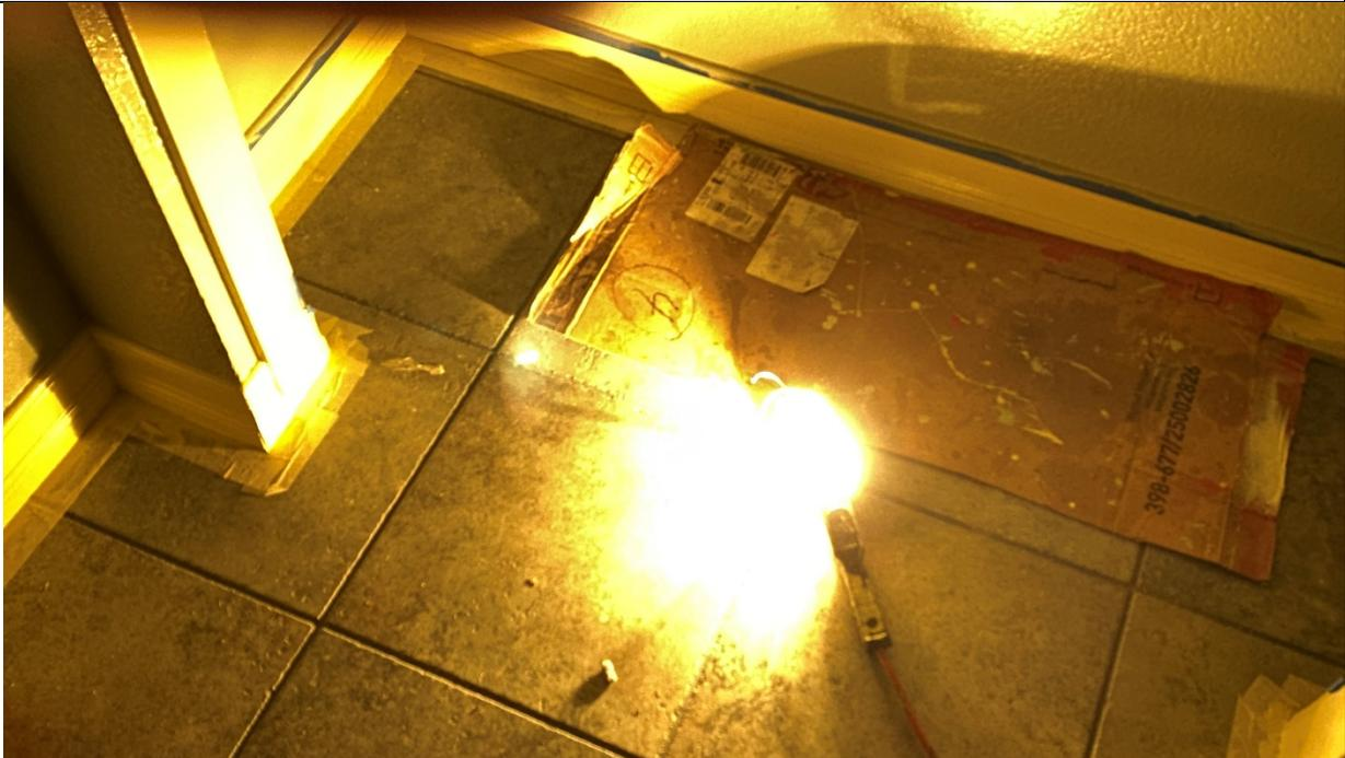
Photo of home 60 W incadescent trouble light for comparison to photos of LED lights – No blue ghosting marks visible.
