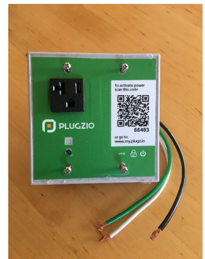
Plugzio is an example of a “smart outlet” that allows a MUD operator to be reimbursed for house power used for EV charging by retrofitting an existing 120v outlet on a dedicated 15 or 20 amp circuit.
