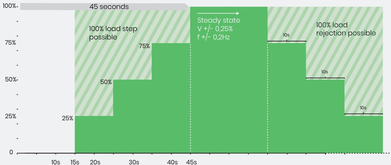
1. Example profile for pre-heated/lubricated; Without synchronization; 480 V configuration; Power quality within +/- 10% voltage, +/- 5% frequency
