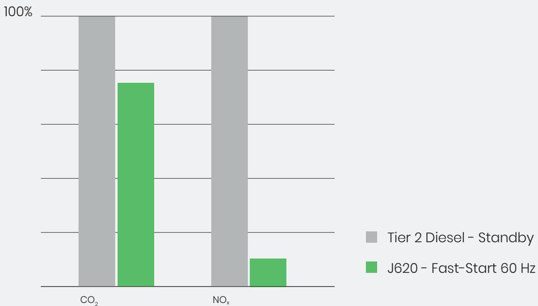
**The Jenbacher J620 fast-start, natural gas generator without after treatment technologies can provide an emission reduction of up to 23% CO<sub>2</sub> and up to 90% NO<sub>x</sub> compared to Diesel Tier 2 standby generators.**
