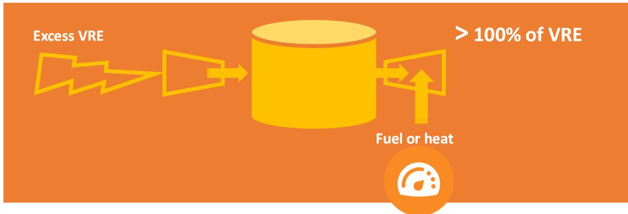
Figure 10. Hybrids use fuel or heat to boost the performance and reduce the cost of energy storage
