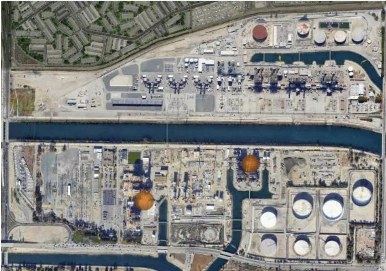
Figure 6. Haynes Generating Stations includes a large fuel oil tank farm in the lower right that could be redeveloped for hybrid thermal energy storage.
