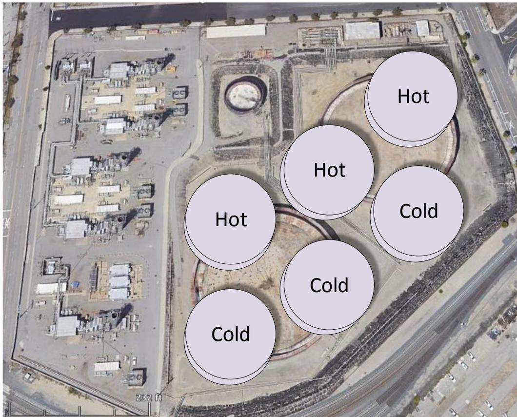
Figure 4. An 11,000 MWh energy storage system could be deployed at Harbor Generating Station, using six molten salt storage tanks, similar in design and construction to the 12 tanks installed at the Solana CSP station in Arizona. Similar systems could also be installed at the Scattergood and Haynes Generating Stations.
