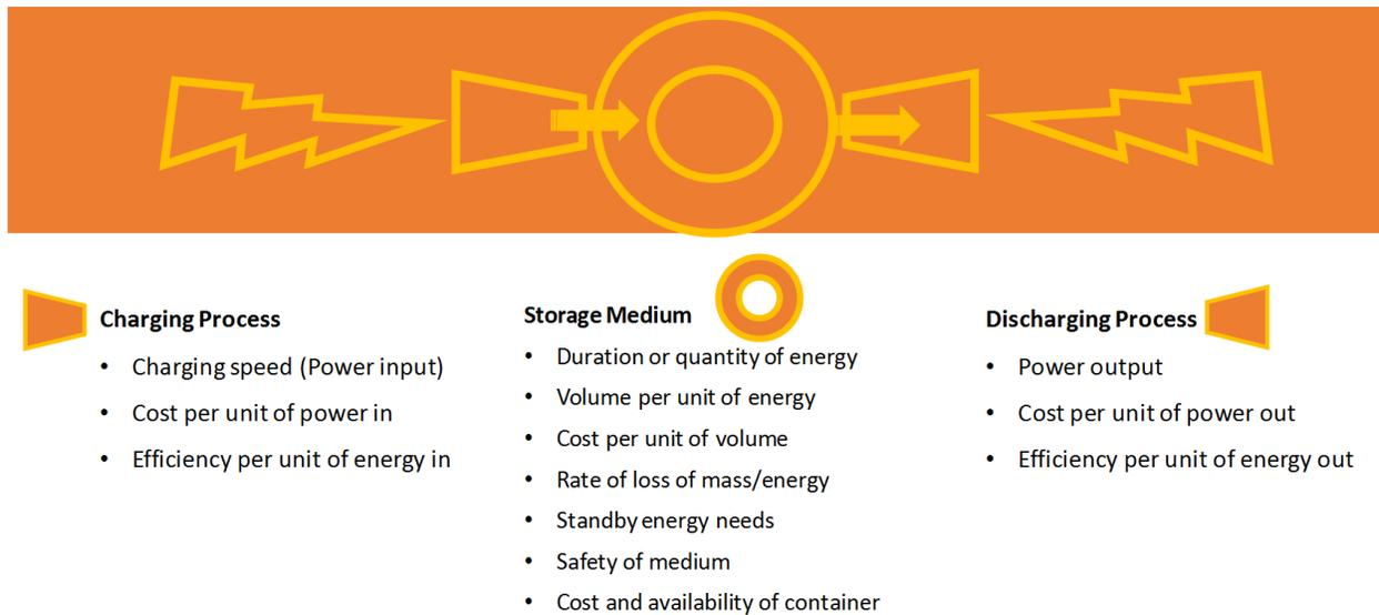
**Figure 8. Electricity must be transformed into internal energy during charging and transformed back to electricity during discharging**
