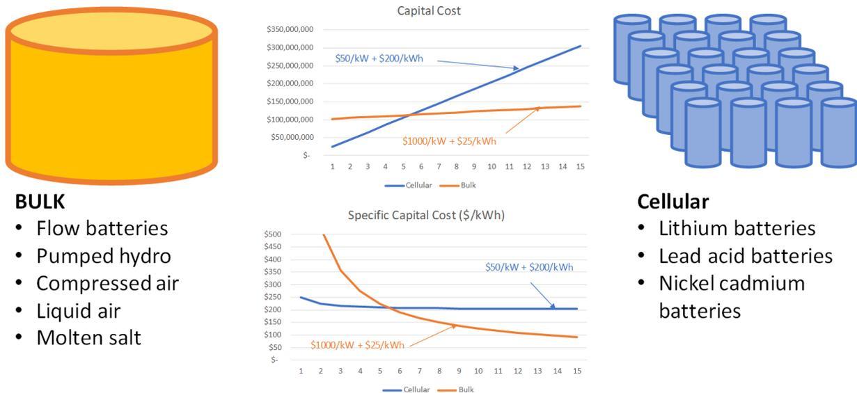
Figure 9. The form factor of the storage medium affects cost and specific cost.
