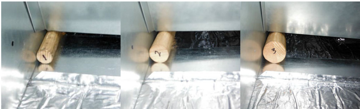
Figure 5: Economizer damper positions using 1, 2, and 3-finger dowels
