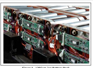
Figure 3 – Lithium-ion Battery Pack
