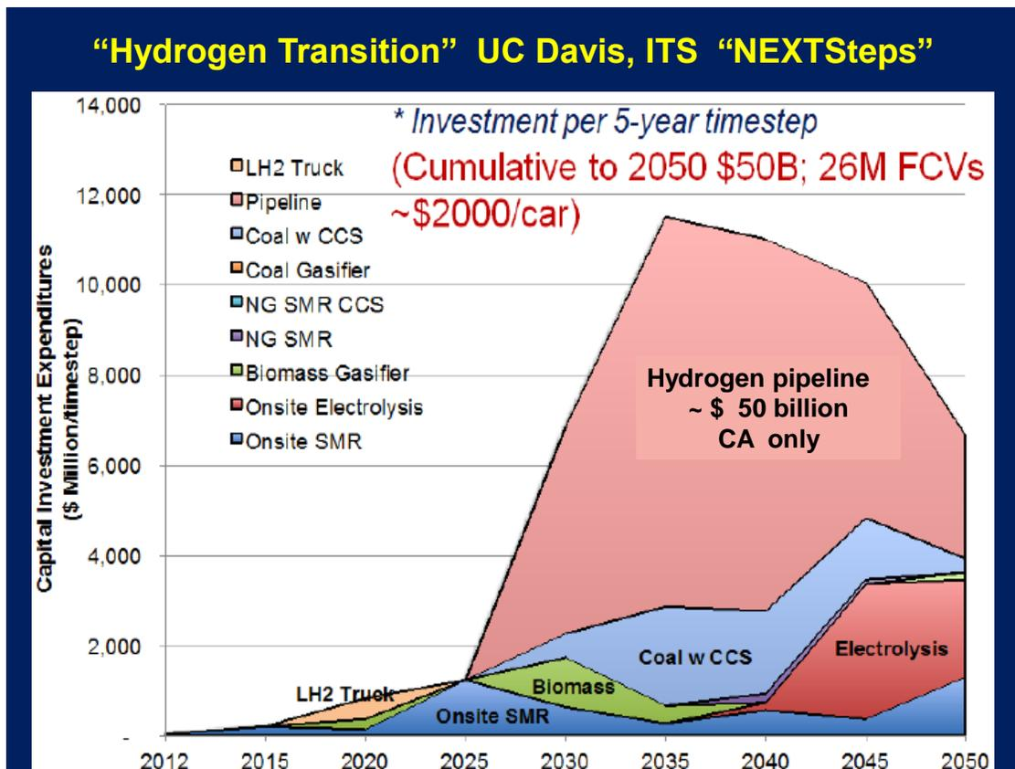
Figure 5. From "The Hydrogen Transition", ITS-STEPS, 2014 <sup>1</sup> Large cumulative capex for "Hydrogen Pipeline" if building a new, dedicated, high-purity, underground GH2 pipeline system ; less capex if diverse extant pipelines are repurposed .
