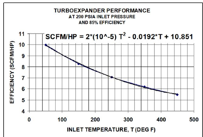
Fig. 9 – Temperature vs. Turboexpander Volume/Power efficiency
