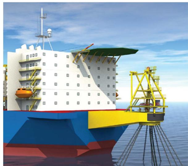
Fig. 3 – Cantilevered Arm with Turret – Courtesy of SBM Offshore
