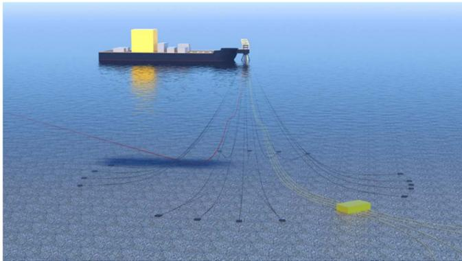
Fig. 5 – The turret mooring spread showing array and export power cables
