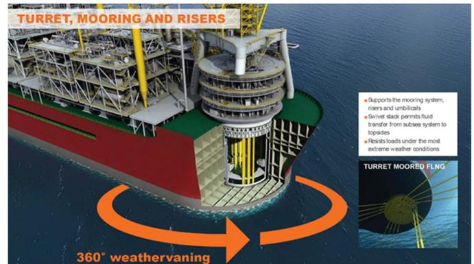
Fig. 2 –FPSO on a turret mooring – Courtesy of SBM Offshore
