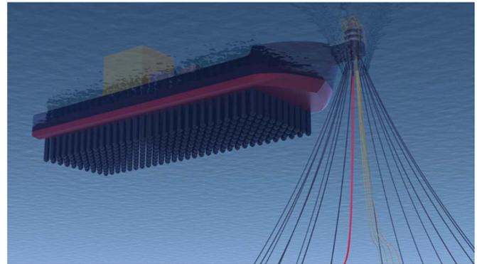
Fig. 6 – Underwater view showing submerged compressed air tanks
