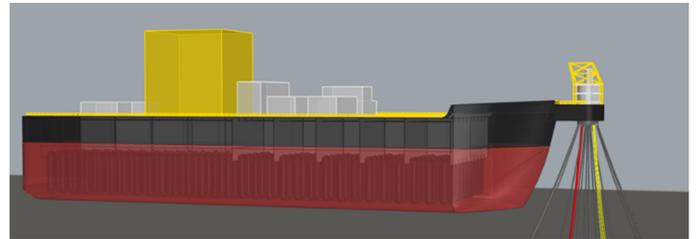
Fig. 11 – Platform option with tanks enclosed inside the hull
