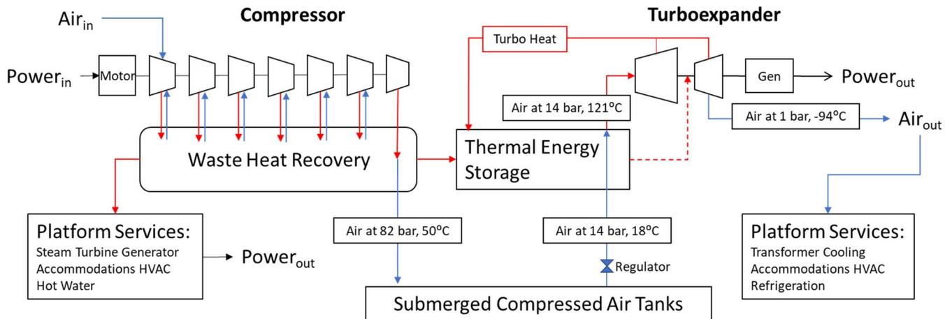
Fig. 8 – CAES-STS System Schematic
