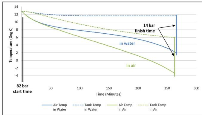
Fig. 10 – Internal air temperature for storage tanks submerged in water vs. air, 13°C (55°F) ambient
