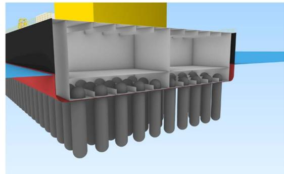
Fig. 7 – Cutaway view showing inner bottom tank spaces
