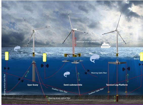
Fiber Optics System for a Real-Time Monitoring
