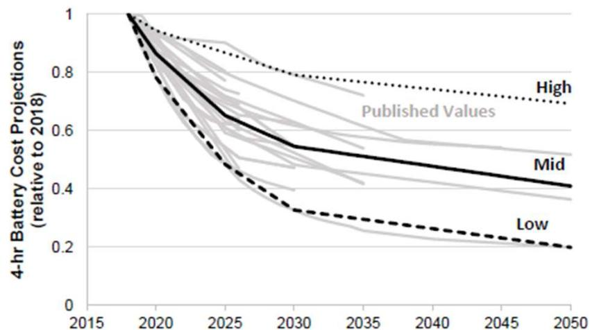
**Figure 1. Battery cost projections for 4-hour lithium-ion systems, with values relative to 2018.** The high, mid, and low cost projections developed in this work are shown as the bolded lines. Figure values are included in the Appendix.
