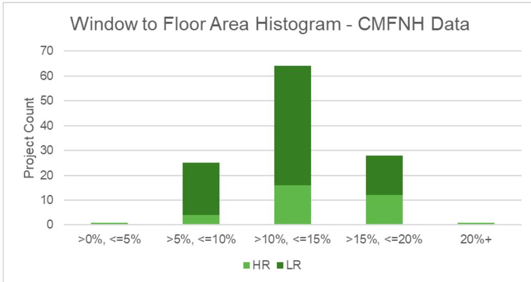
**Figure 5: Window-to-floor area histogram – CMFNH data.**
