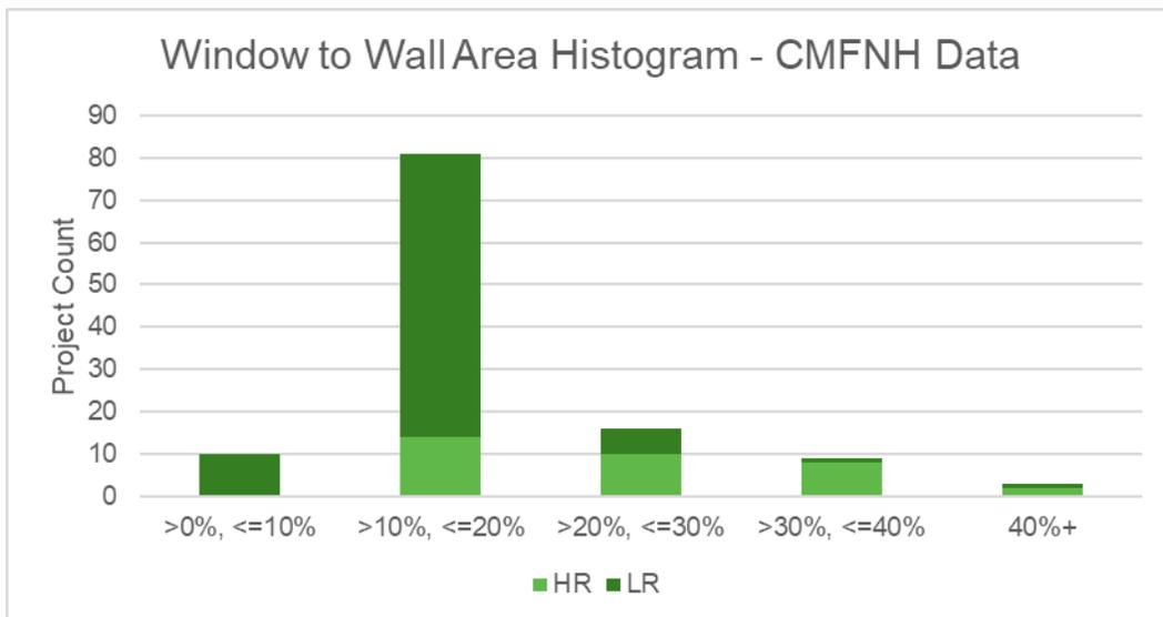
**Figure 6: Window to wall area histogram - CMFNH Data.**
