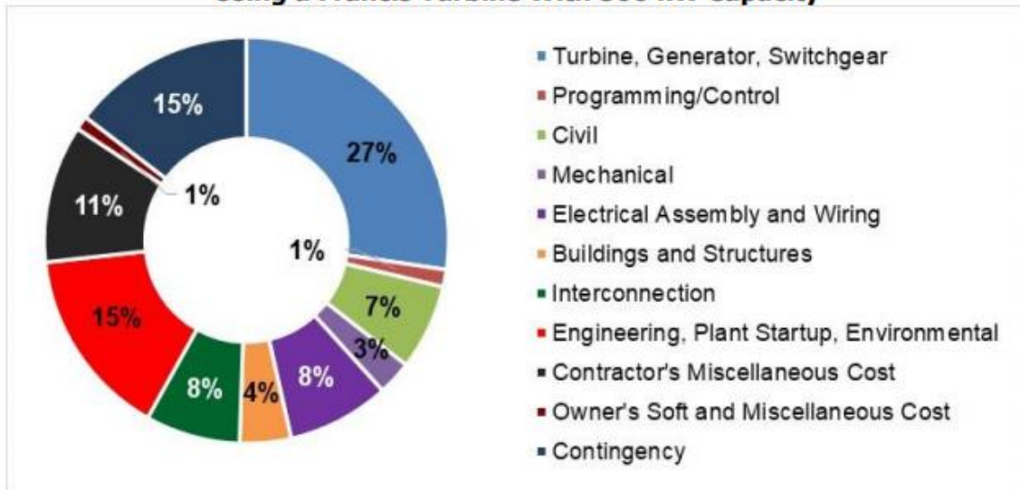
Figure ES-1: Example of Capital-Cost Breakdown of In-Conduit Hydropower Project Using a Francis Turbine With 500 kW Capacity
