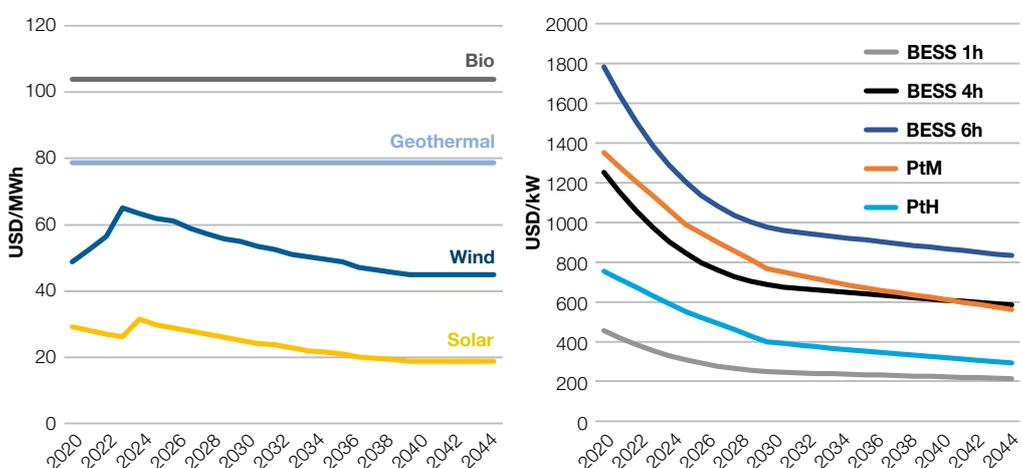
**Figure 13.** Levelized Cost of Energy for Renewable Energy Sources (left) and storage technology price (right) learning curves. Source: IRP dataset, Bloomberg NEF Source: IRP dataset, LUT.
