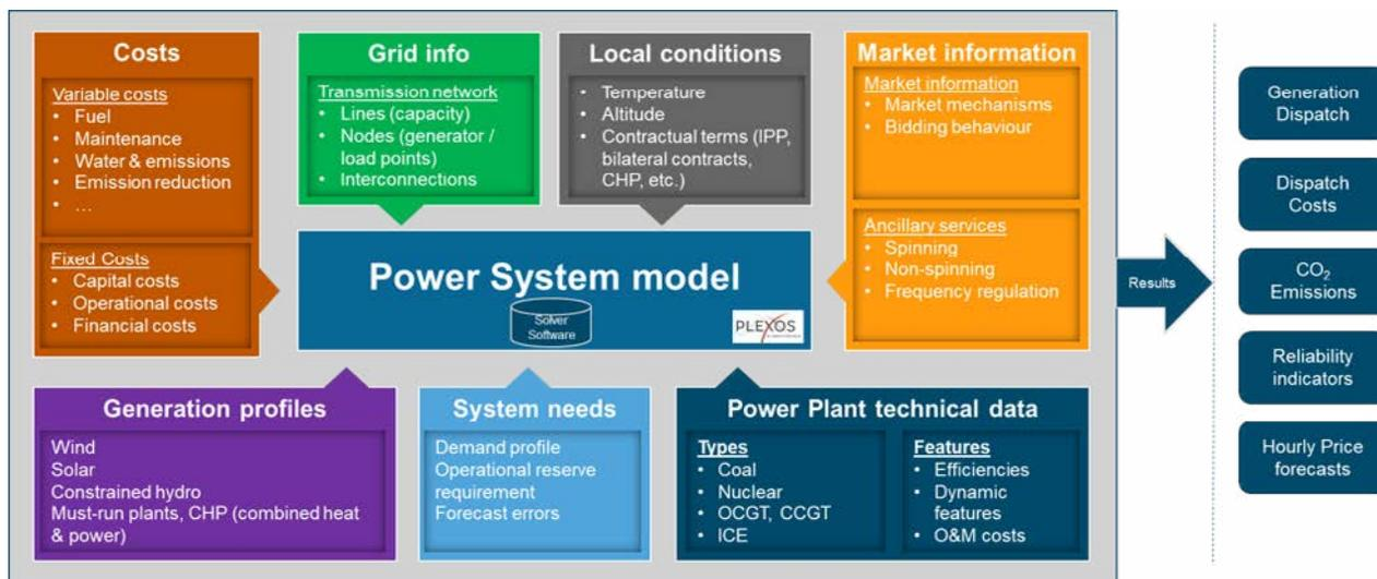
**Figure 14.** Plexos power system model (requires major computing power).
