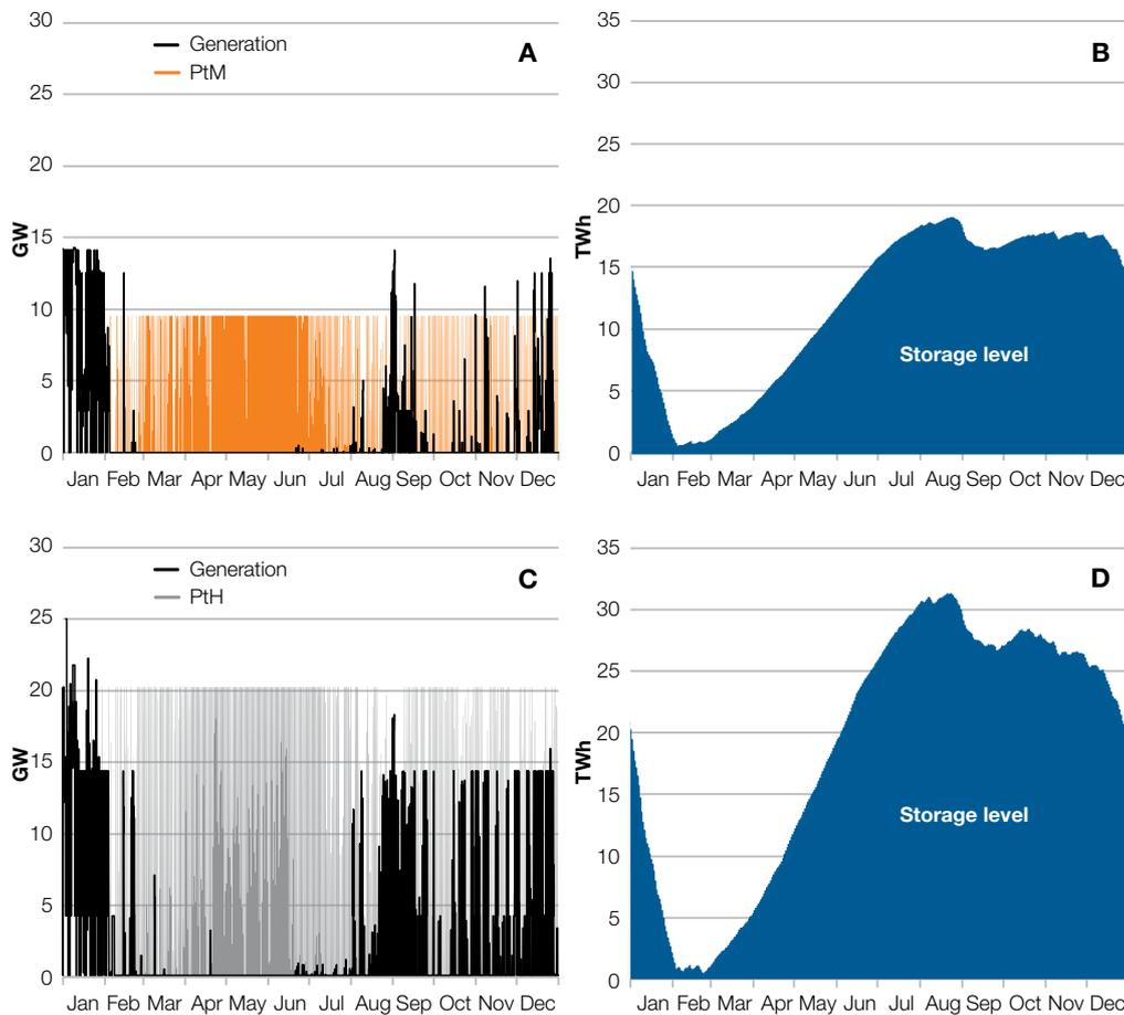
**Figure 8.** Power-to-gas (PtG) utilization in 2045, Optimal Path. Annual hourly thermal generation and electricity consumption (GW) of PtM and PtH (panels A & C respectively); Annual storage levels of renewable gas from PtM and PtH (Panels B & D respectively).
