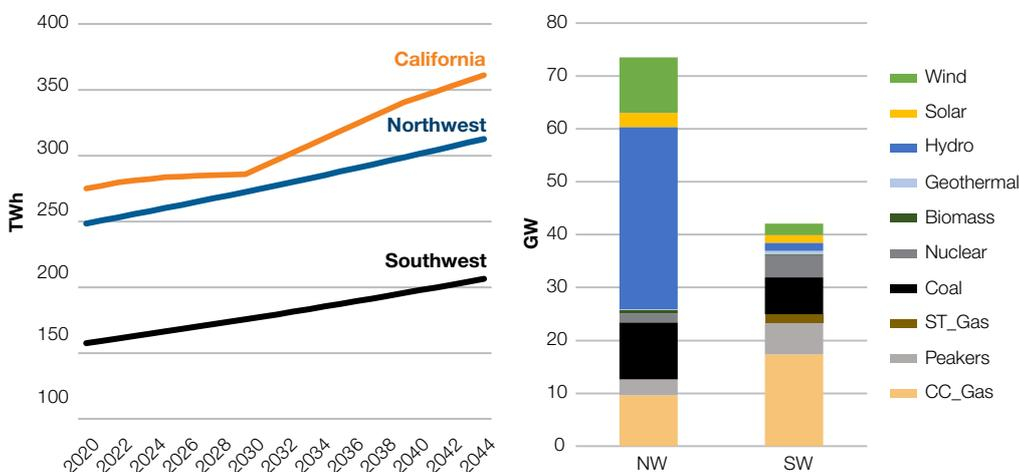
**Figure 12.** Electricity demand by regions (left) and Initial Installed capacity in NW and SW Regions (right).
