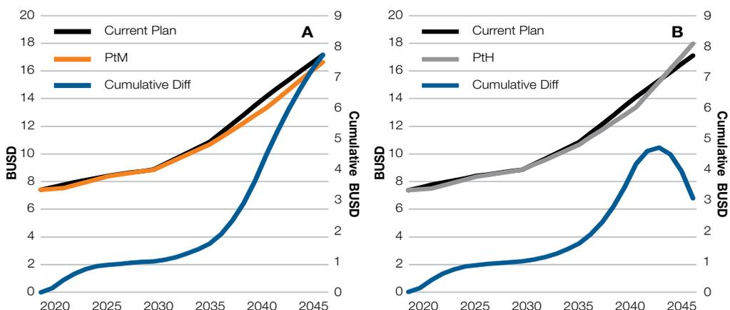
**Figure 7.** Annual total generation cost of Optimal Path and Current Plan, and cumulative savings of Optimal Path versus Current Plan via PtM (A) and PtH (B). Note: 2020 cost is only OpEx while the cost after 2020 includes both CapEx and OpEx of the new investments.
