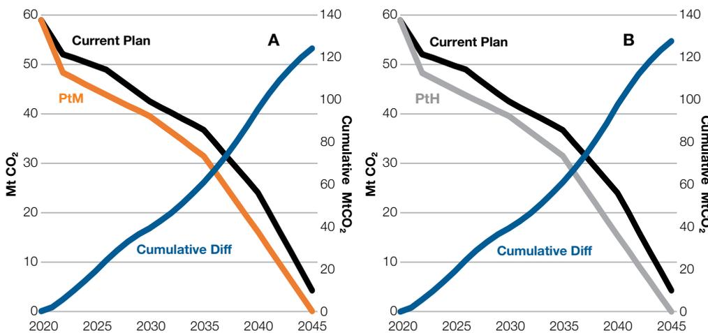
Figure 4. Annual CO<sub>2</sub> emissions for Current Plan and Optimal Path PtM (A) and PtH (B) across 2020-2045, and the cumulative emissions savings with Optimal Path.
