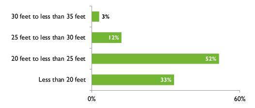
Figure 12: Typical mounting height for parking poles (n=33).
