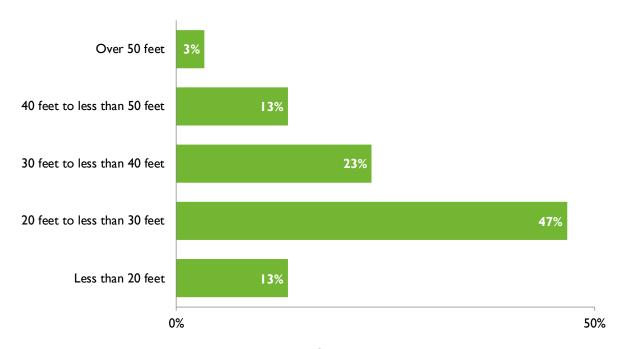
Figure 16: Typical pole to pole spacing for pedestrian poles (n=30).
