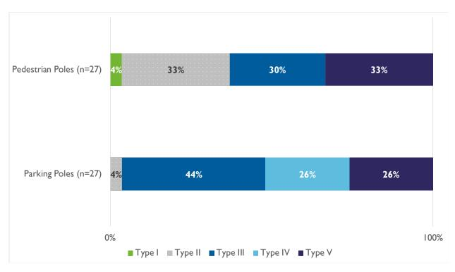
Figure 20: Typical light distribution for pedestrian and parking poles for projects completed in past six months.
