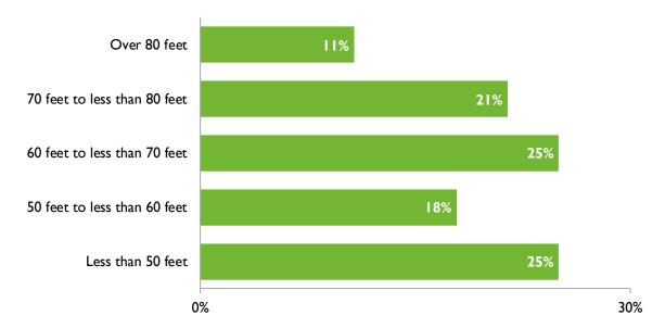
Figure 15: Typical pole-to-pole spacing for parking poles (n=28).
