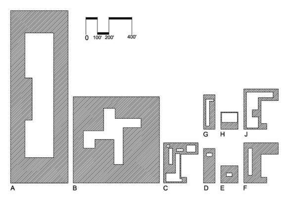
Figure 1: Representation of general hardscape layouts used to determine new lighting power allowances.
