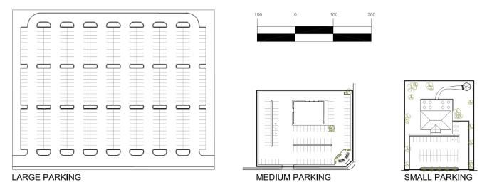
Figure 2: Real parking lot designs used to confirm recommended light levels could be achieved with the proposed lighting power allowances.
