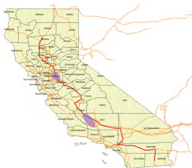
Figure 60. Map of potential CO 2 trunk pipeline. California counties are shown with existing major natural gas pipelines in orange. Approximate proposed CO 2 storage areas are marked with purple ovals. The base case CO 2 pipeline is shown in red. This route follows major natural gas pipelines and passes through our studied storage sites in the central valley, and a potential geothermal-powered direct air capture plant near the Salton Sea.
