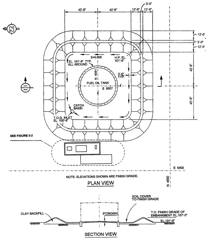
Figure 4-2 Fuel Oil Bulk Storage Tank
