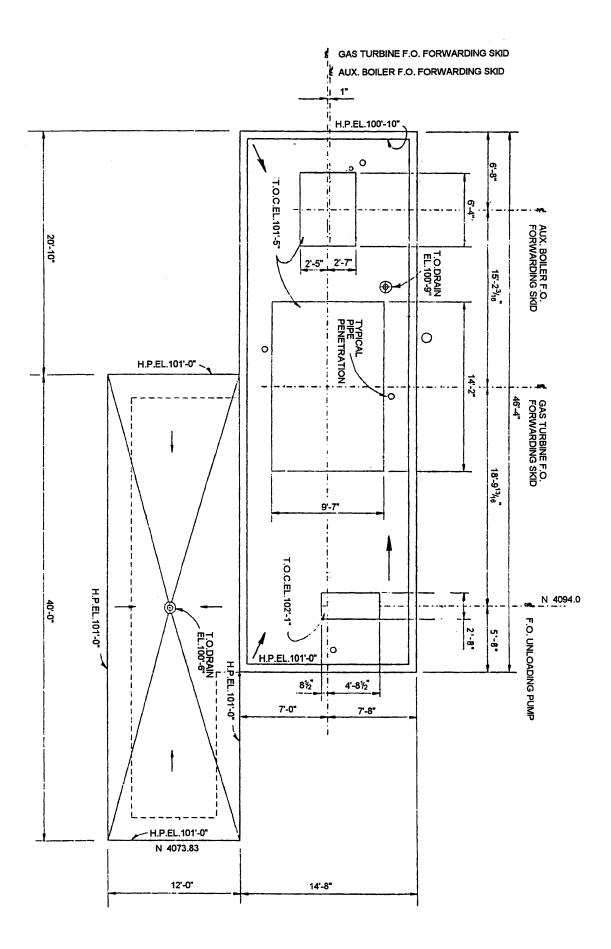
Figure 5-2 Fuel Oil Forwarding Area Secondary Containment
