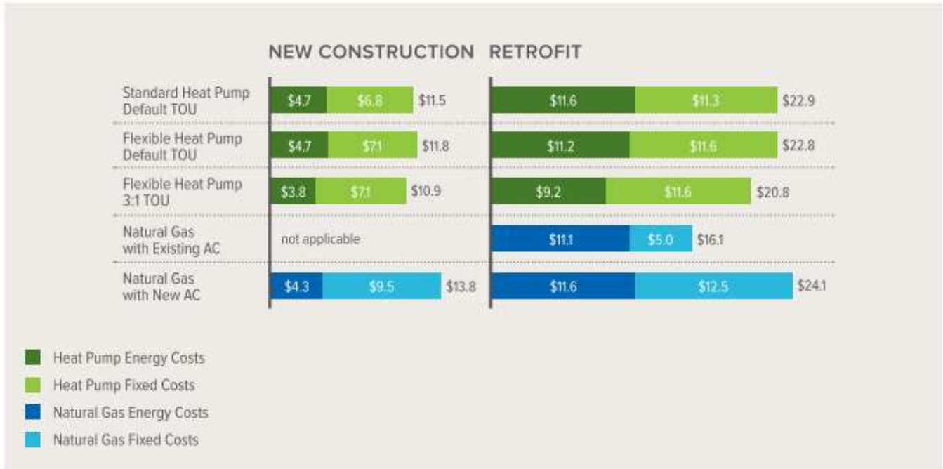
Figure A-1: Heat Pump vs. Natural Gas Furnace Lifetime Net-Present Cost Comparison (Oakland, California)
