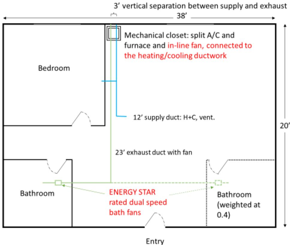
Figure 24: Base case: discrete supply in-line fan.
