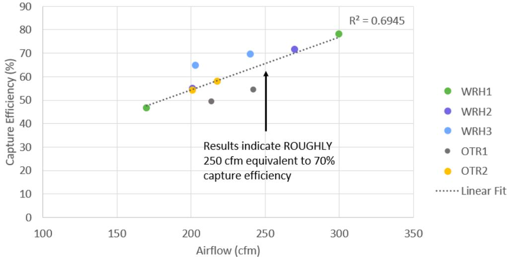
**Figure 16. Capture efficiencies of example undercabinet and microwave range hoods.**
