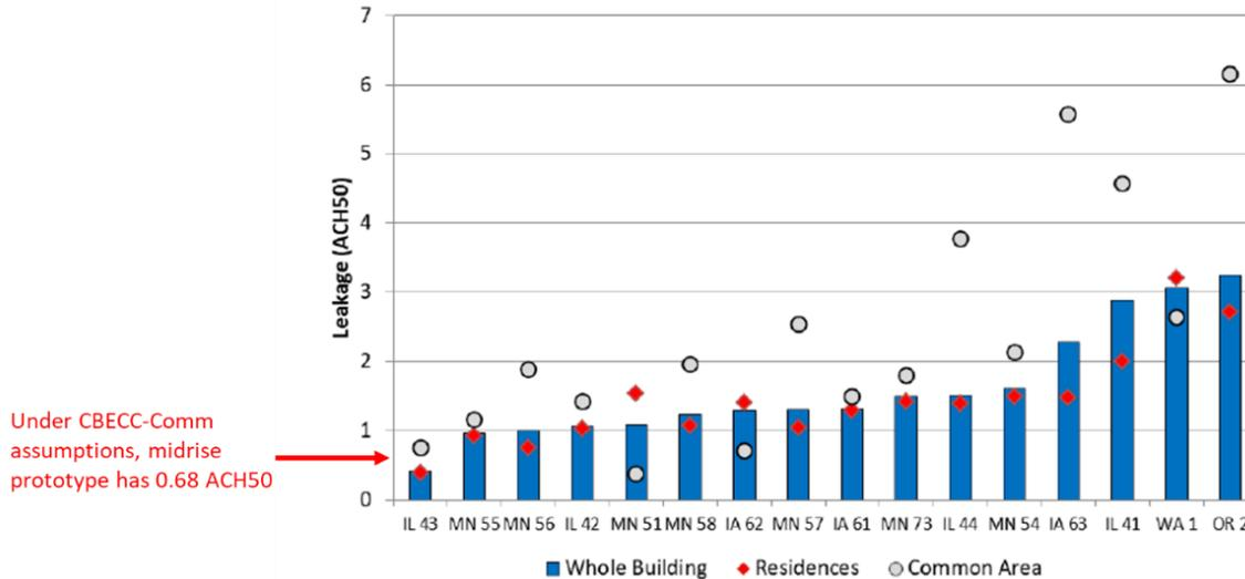
**Figure 32: Multifamily leakage (measured at the whole building level) compared to CBECC-Comm infiltration assumption**
