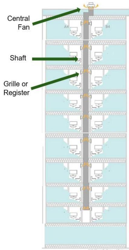
**Figure 11. Diagram of central ventilation duct system components.**
