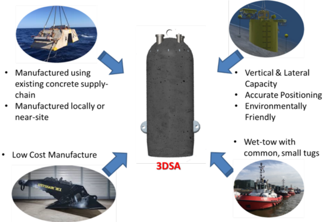
Figure 2. The 3DSA is designed to take advantage of the positive aspects of other anchoring concepts (low-cost, accurate positioning, quiet installation and omnidirectional load capacity) whilst mitigating high-cost items (logistics and installation) and reducing installed CapEx by 80%.
