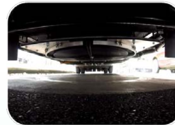
Wireless Advanced Vehicle Electrification (WAVE) Inductive
