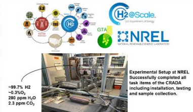
Fig. 3 TRL 4 GTA electrolyzer that was used for testing and validation at the National Renewable Energy Laboratory. In addition to the electrolysis cell, the pressure regulators and electronic control equipment that were used to operate the system are also shown. The sample collection cylinder is in the foreground. Gas samples with and without an oxygen scrubbing step were collected and sent to SmartChemistry, Sacramento, CA for purity analysis. As discussed in the Results section, the native hydrogen purity was sufficient for almost all the hydrogen industrial operations shown in the upper left graphic.
