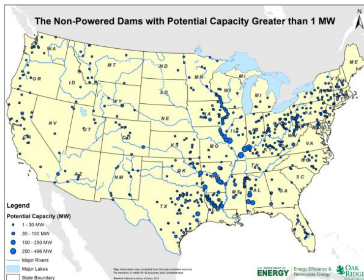
Figure ES-1: Locations of the top non-powered dams with potential hydropower capacities greater than 1 MW
