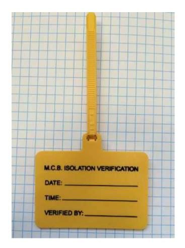
Attachment 1 – Molded Case Breaker Isolation Verification Tag
