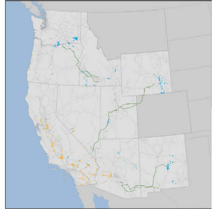
Full West Siting Level 3 (Constrained) ■ Solar Selected Project Area ■ Wind Selected Project Area ■ Interconnection — Planned Transmission — Existing Transmission
