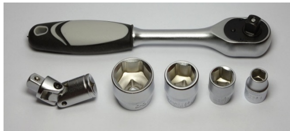
Figure 15: Socket wrench, universal joint and sockets. Picture by Kae, CC BY-SA 3.0
