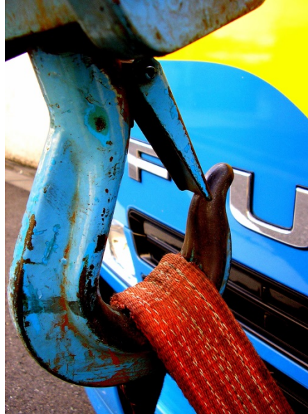
Figure 10: crane hook with a safety latch closed. Picture by tanakawho, CC BY 2.0
