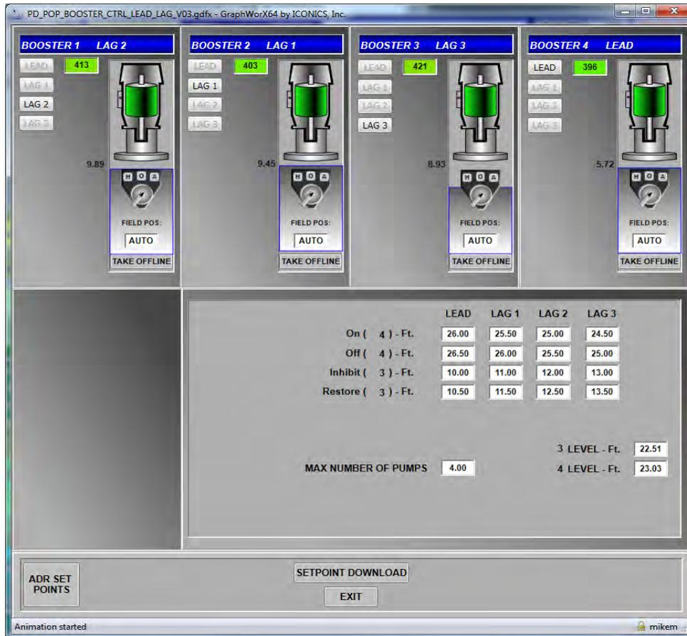
Figure 7. CVWD SCADA Lead/Lag Settings Based on kWh/AF<sup>19</sup>
