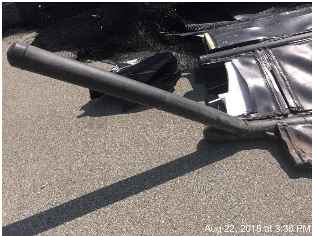
Detail of the leak detection piping system, as removed from MCWP No. 1 and 2.
