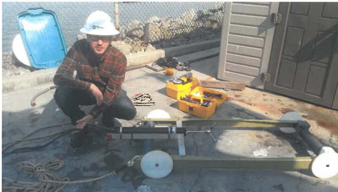
Figure 2-5. Nortek Vector Acoustic Doppler Velocimeter (ADV) mounted on a sled in a horizontal pointing direction prior to measure intake approach velocities at the Moss Landing Power Plant Units 1 & 2 intakes.
