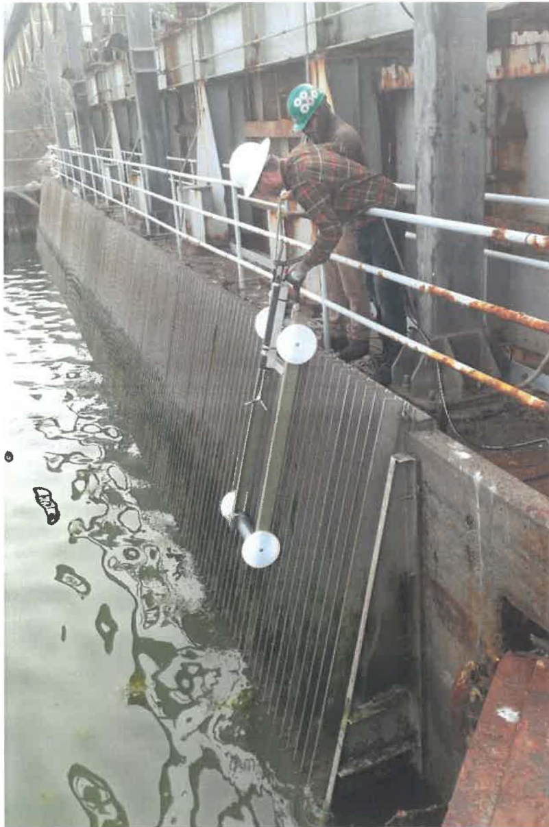
Figure 2-6. Deployment of the Nortek Acoustic Velocimeter (ADV) at Units 1 & 2 intake structure during the 2018 approach velocity measurement survey.
