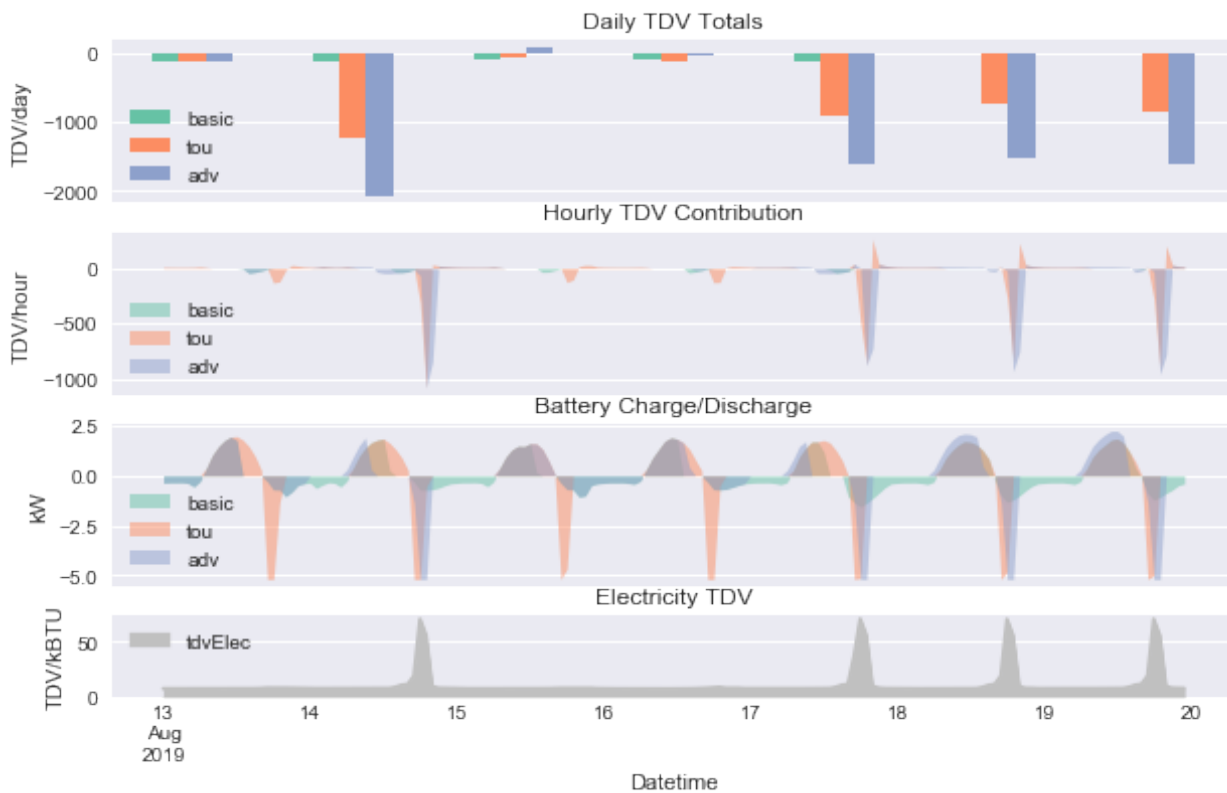
Figure 3: On days with high Electricity TDV, the TOU and Advanced control strategies can accumulate large negative TDV by discharging to the grid during peak hours. The Advanced strategy specifically targets the top three TDV hours each day for discharging.
